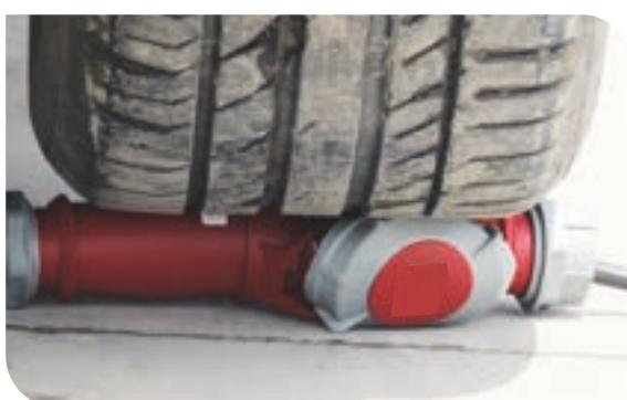
We designed and developed products, mainly to meet the long-term work in the exposed environment. So that the product has better, better compression capacity. Our test in order to facilitate the real environment in the test, to enrich the performance of product design and development.
